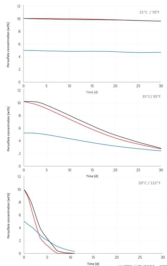
Storage Stability of Aqueous Persulfate Solutions at Different Temperatures (APS / NPS: 10% solutions: KPS: 5% solutions: temperatures = 21, 35, 50 °C
